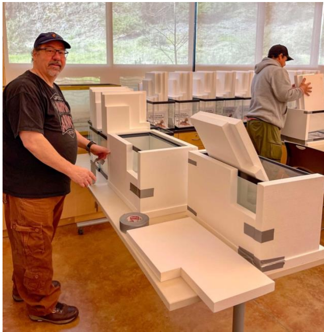
Allen Espinosa and David Berman attaching Styrofoam insulation blocks to the outside of the glass steelhead egg tanks.
